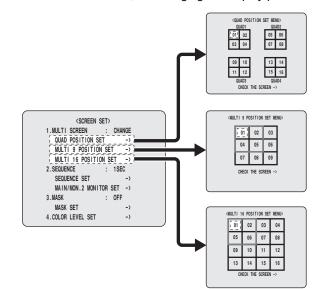
Example: Switching the live video of the camera 5 and camera 1 on the quad screen.
